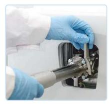
With DIP option, you can utilize the MS as stand-alone by injecting liquid or solid samples directly into the MS. Switching from GC/MS injection to DIP/ MS injection takes only a couple of minutes.
