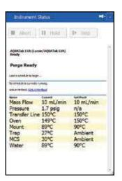
**Instrument Status Screen** - The Instrument Status screen provides valuable information such as mode operation and instrument conditions. During Leak Check, it displays the region of the system that is being checked and the time remaining of the leak check.
