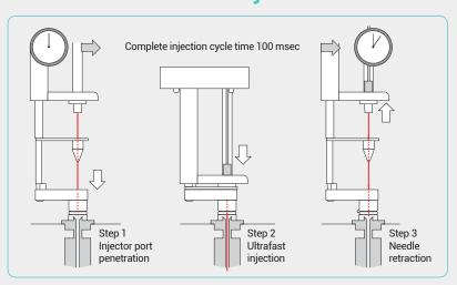
Ultrafast injection down to 100 msec reduces needle discrimination in GC to C40/C20 > 0.98.
